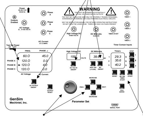
The selected parameter can be set using the control knob or the Increase or Decrease buttons. In some cases the buttons give finer control than the knob.
